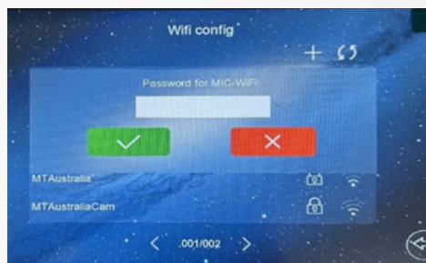
5. Enter the password for the 2.4 GHz WI-FI and press the tick to save. You will know the connection is successful when the WI-FI symbol is solid.
