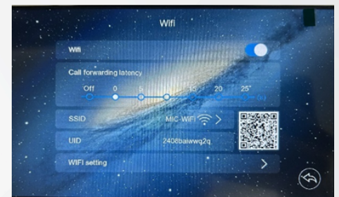
3. Press on the > alongside SSID, this will now start scanning for the 2.4GHz WI-FI
